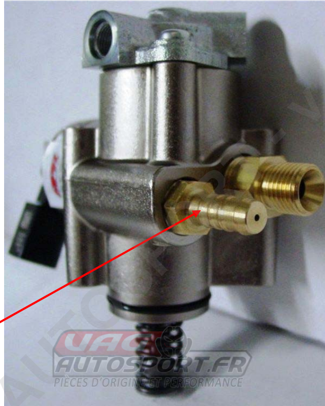
FIG 2: FSI Fuel Pump shown with “Bamboo” type fitting where a hose is pushed-on to the barbed fitting and secured with a hose clamp.
