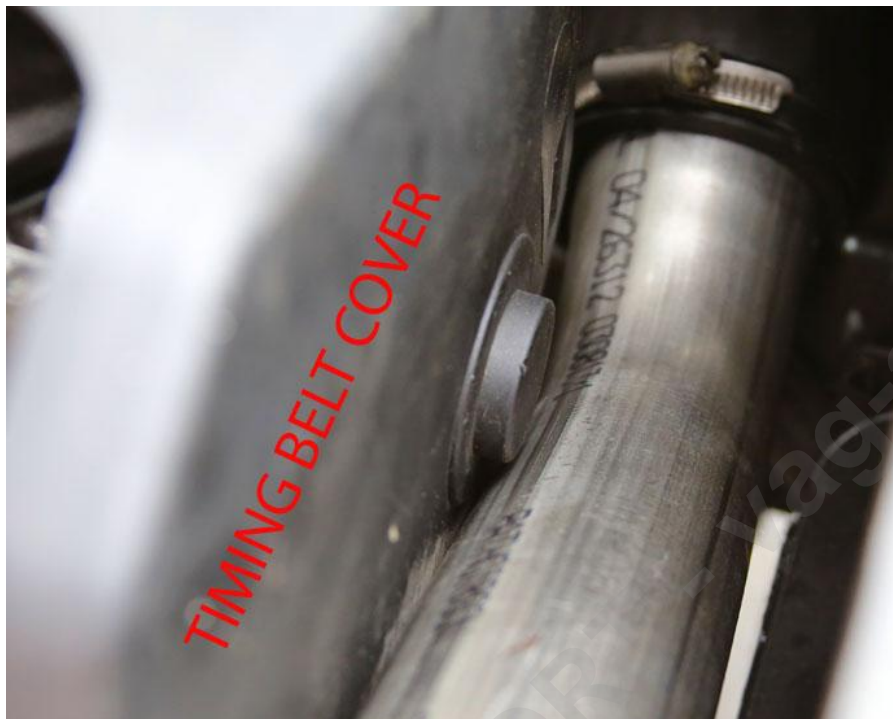
Driver side Bi-Pipe Installed
